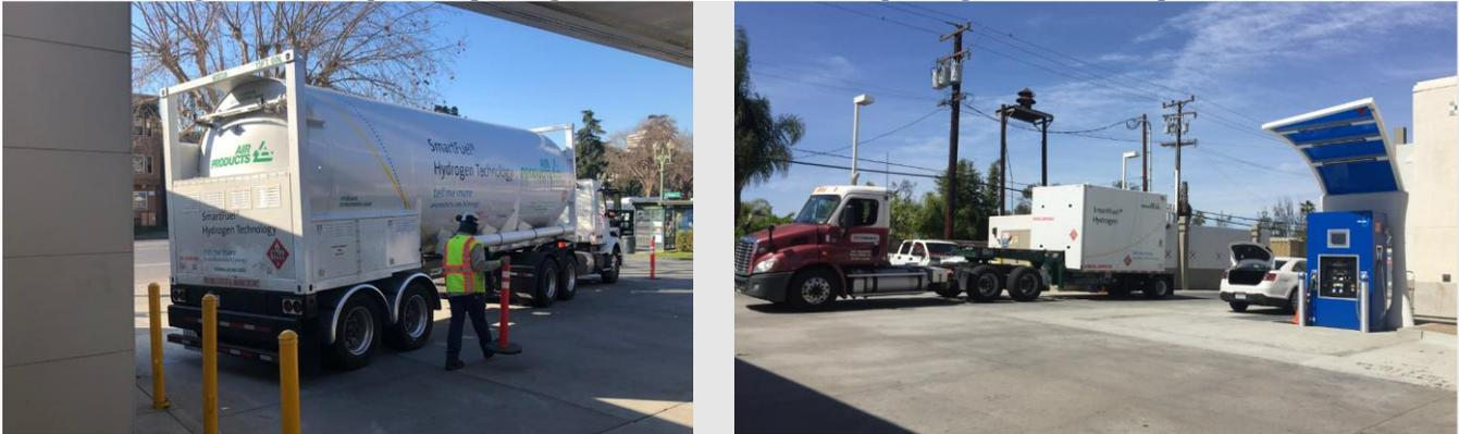
Liquid hydrogen truck can deliver 2,400 kg (left) compared to 120 kg for gaseous hydrogen truck (right).
