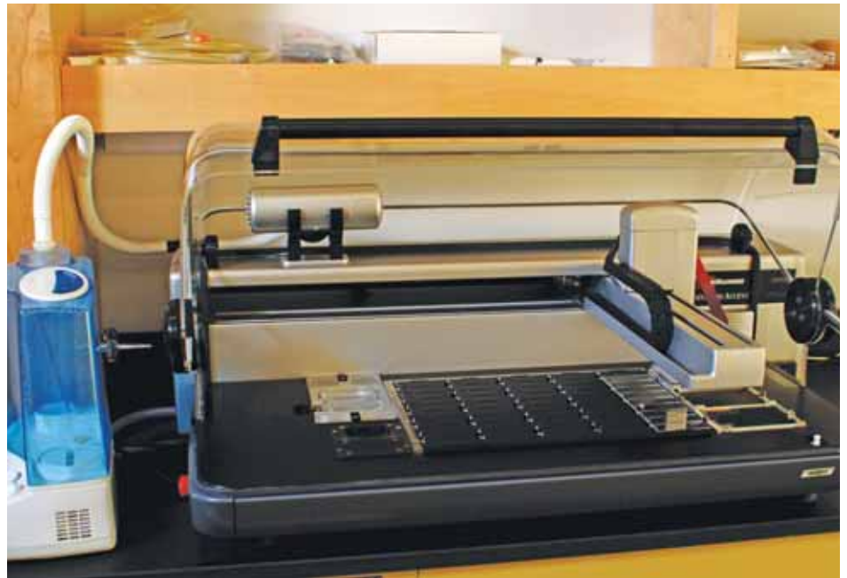
ABOVE: The Omnigrid microarrayer makes microarrays—spots of DNA on a glass slide—that are used in the genomics research that underlies the study of Streptococcus pyogenes in the Bessen microbiology laboratory.
